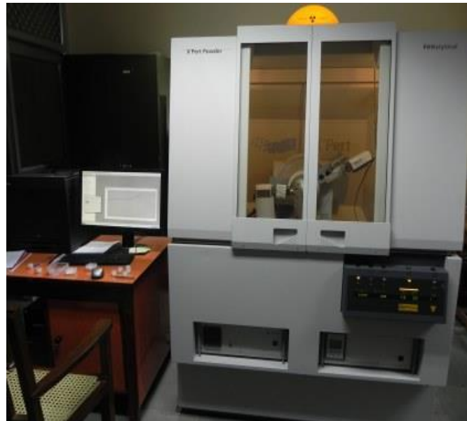
Figure 3.2 Powder X-Ray Diffractometer
