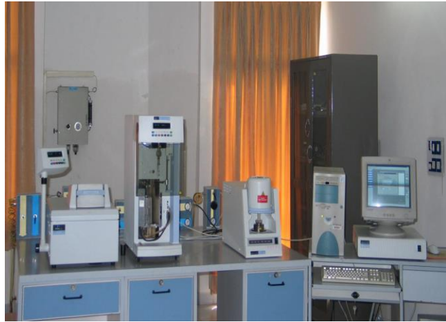
Figure 3.3 Instrumentation of TG-DTA
