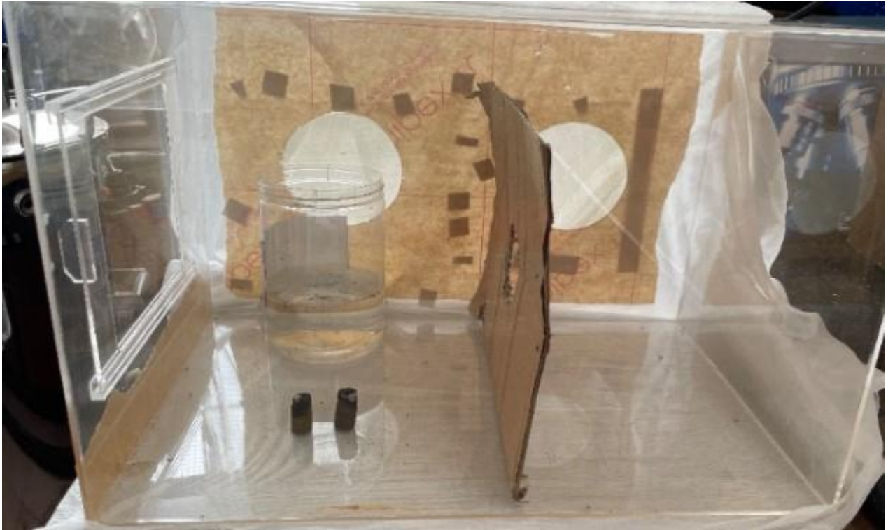
Figure 23 Excito-chamber test for Aedes spp
