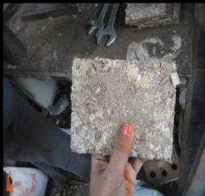
Sample made of willow waste with water hyacinth
