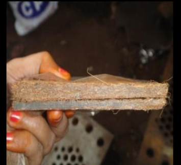
Both the above are samples made of (willow waste + coir)
