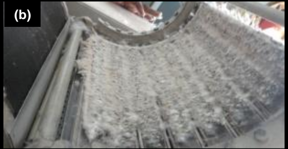
Accumulated trash inside the combing machine during web formation
