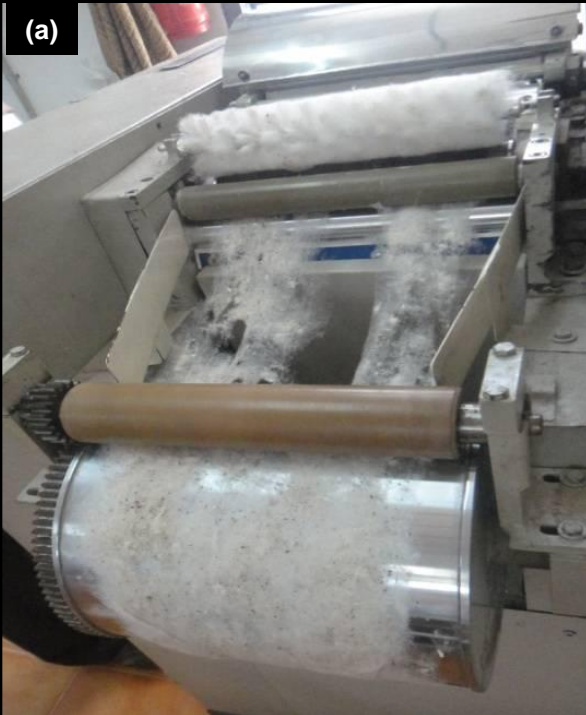
(a) The web obtained from willow waste
