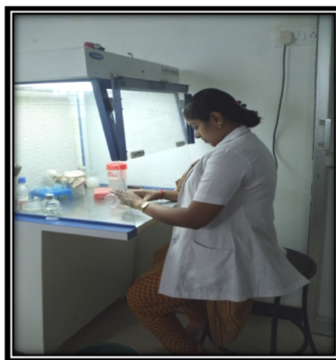
Assessing Microbial Count in Lamina Air Flow Chamber
