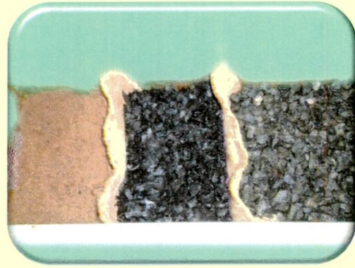
9b. GCS Filter with Nonwoven Agave americana -Hemp Screens
