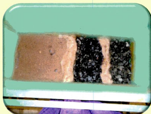
10e. GCS Filter with Nonwoven Agave americana -Hemp Screens in Proportion 1:2:3
