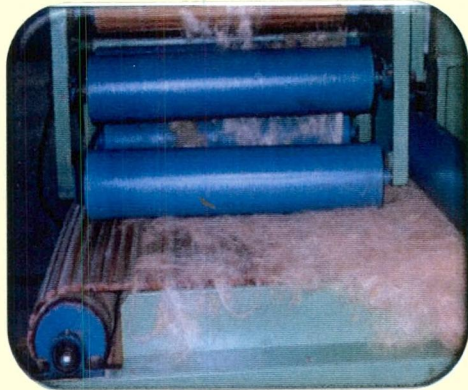
5a. Cross Lapping of the Web in the Finisher Card
