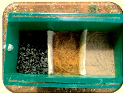
9f. Gravel / Coir Fibres Sand with Woven Hemp- Agave americana Screens
