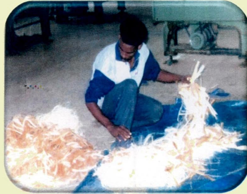
4b. Mixing Fibres for Hand Batching
