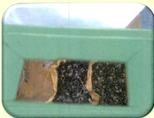
9e. GCS Filter with Woven Agave americana -Jute Screens
