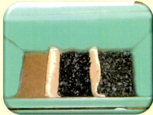
9d. GCS Filter with Nonwoven Agave americana Screens
