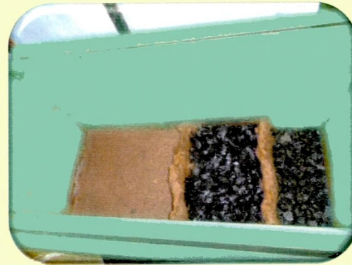
10d. GCS Filter with Nonwoven Agave americana -Jute Screens in Proportion 1:2:3
