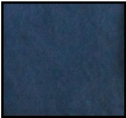
f, Fabric dyed with reactive dye navy blue GDB using fresh water
