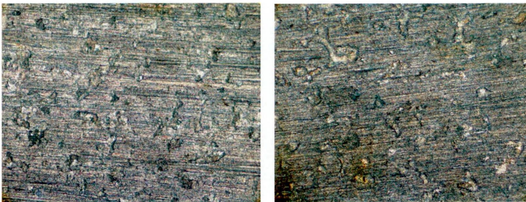
Photomicrographs of MS in presence of L.S.E. (25b) and in presence of S.F.E. (25c)
