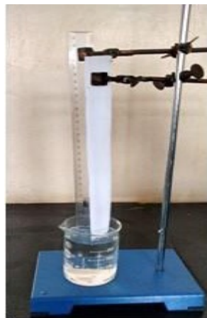
Plate-XV Vertical Wicking Test
