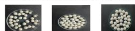
Fig. 4. Diatomaceous Earth Balls formulated at different concentrations at 0.5g, 1.0g, and 1.5 g
