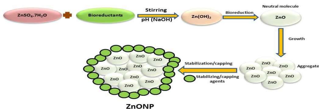
Figure 22. Proposed mechanism of formation of ZnONP
