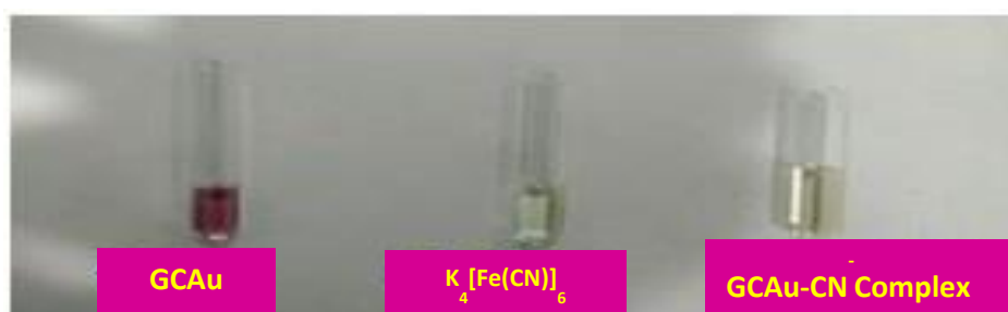
Figure 74. Colour change of GCAu when reacted with CN - ions
