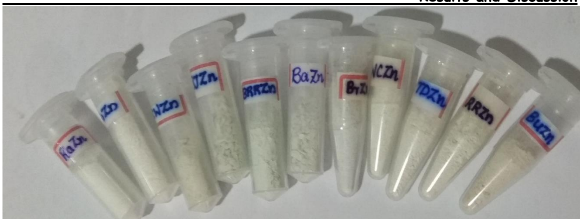
Figure 21. Synthesized ZnONPs using cereals and pulses washed water
