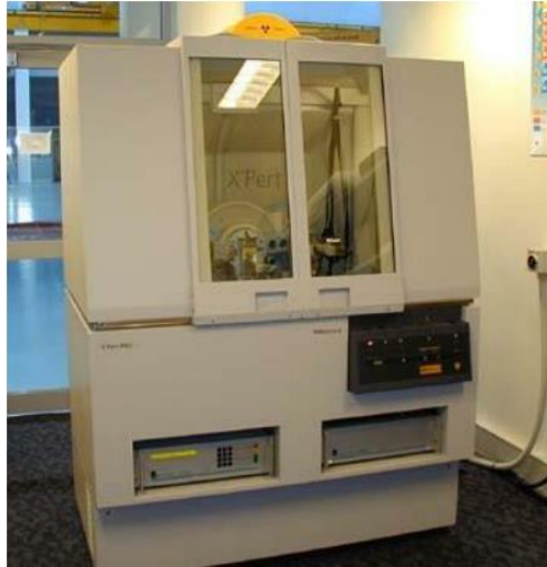
Figure 3.3: Powder X-Ray Diffractometer instrument
