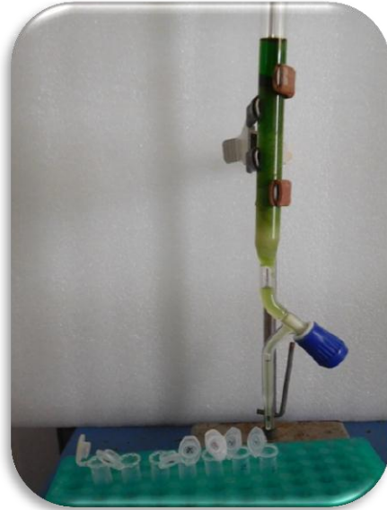
Plate 6c – Separation of Bioactive components in methanolic extract of Passiflora edulis using Column Chromatography
