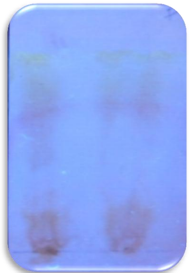
Plate 7b – Distance travelled by the components present in methanolic extract of Passiflora edulis in paper chromatography
