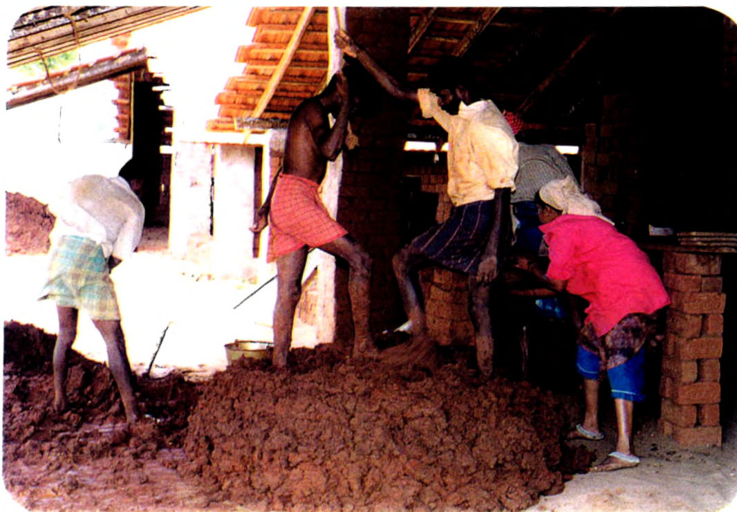
MEN IN MIXING CLAY AND SAND FOR MOULDING BRICKS
