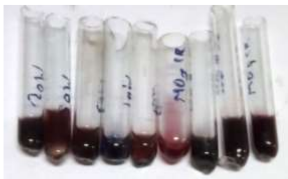
Figure 10. Photograph of synthesized gold nanoparticles using CRablank by Microwave heating method
