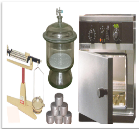
Plate VII Moisture Content Test
