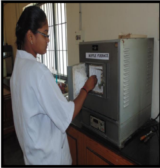
ASHING IN MUFFLE FURNACE
