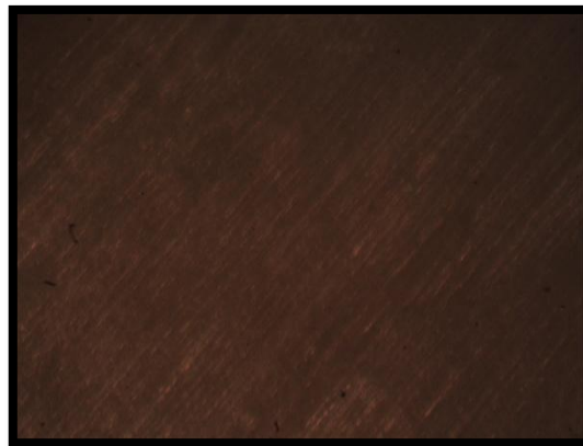
(c) PHOTO MICRO GRAPH OF MS IN CSS/1M HCl
