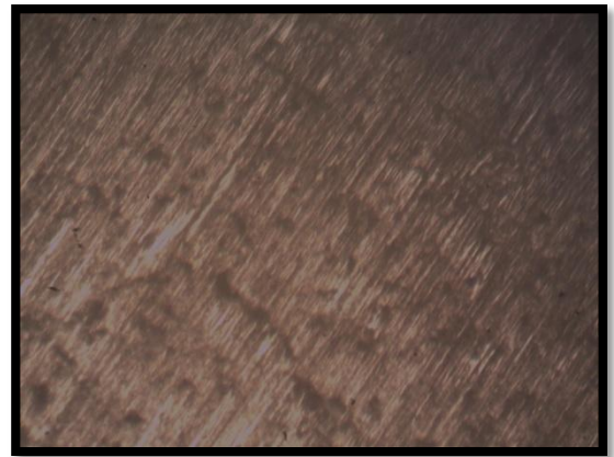
(b) PHOTO MICRO GRAPH OF MS IN THE PRESENCE OF HCl
