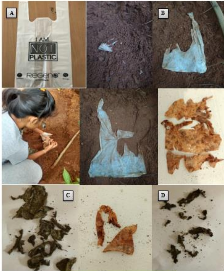
A. Biodegradable bags Biodegradable bags degradability in soil B. After one month C. After two months D. After three months
