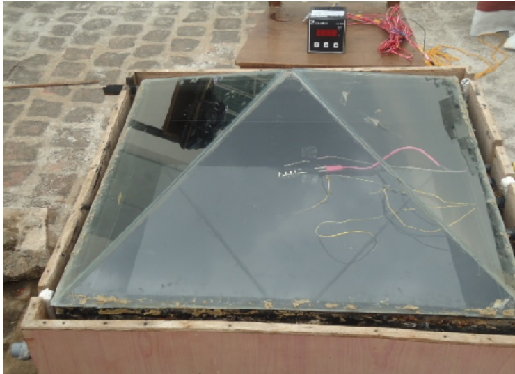
Fig (3.6) Experimental Set Up of the Pyramid Solar Still With Electrical Temperature Controller
